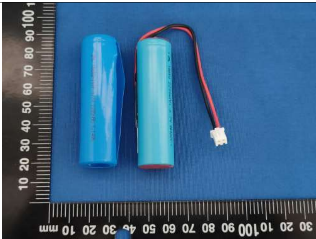
Picture 4 Overall view of Lithium Rechargeable Battery with heat-shrinking tube disassembled
