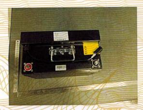
8-LFP-60-EV-NOB Type: 25.6V Rate Voltage: 60Ah(1500Wh) Rate Capacity: Designation: IFpP/330/170/272/[8S3P]M/-20+45/80 17.5kg Weight: 5°C-45°C Chargeing Temperature: Manufacturer Huafu (Jiangsu) Luthium Battery High Technology Co., Ltd. Address Battery Industrial Park of Gaoyou City, Jiangsu Province CE X & A
