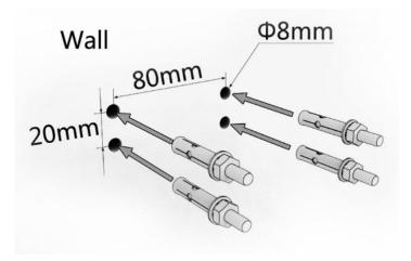
**STEP 3:** Installer the heater on the wall.
