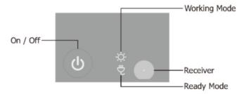
• When the switch is on the **(ON)** position, press the **()** on the panel control . Press it once, the heater will be on 1500W power. Press it again, the heater will be on 3000W power. Press it third time, the heater will be in standby mode.
