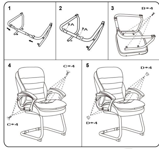
Insert and loosely tighten all screws. When assembly is completed, fully tighten all screws before using. This chair is only intended for sitting. Any other use will void the warranty.
