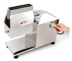
2. Lift up the shield by pulling up the knob.
