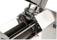
4. Remove the blade attachment. Wear cut-resistant gloves since the blades are sharp.
