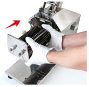
4. Turn the wrench tool to adjust the shafts of blades into firing position.
