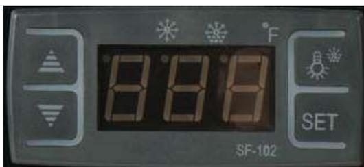
5) Press “▽” for 10 seconds until the display shows “OFF” – this will lock your settings in place.
