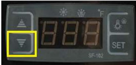
6) Press “SET” again. The display will flash the temperature at which the compressor currently cycles off. The compressor will kick on approximately 7-8 degrees above this set point.
