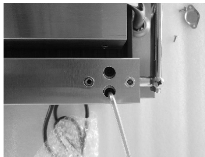
Step 2 - Using an Allen wrench, adjust the tightness to feel. Open and shut the top shell until the tightness feels natural while opening closing the lid. Your manual bag includes this tool. Add any food-safe grease while moving the top shell to lubricate the hinge.
