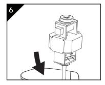
Lower the new motor assembly into the housing by guiding the spindle through the hole.
