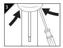
Use a screwdriver to remove the two screws from the top cover.
