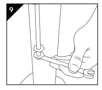
Secure agitators to spindle using a wrench.
