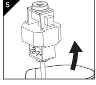
Lift the motor assembly straight up and out of the housing.
