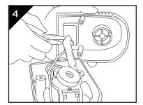
Unplug the blue wire that connects the motor and the top cover housing
