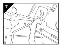
Plug the new motor into the top cover and housing just as it was before **Step 3.**
