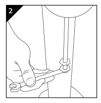
Remove the agitators from the spindle using a wrench.
