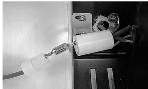
Disconnect the metal locking connectors by squeezing the metal tab.
