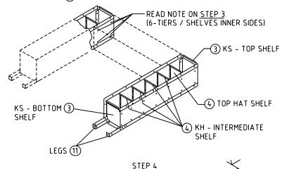
BOLT DOOR AND FRAME (5) ASSEMBLIES TO KS (3) SHELVES AND KP (2) SIDE PANELS STAND UNIT UP AND ALIGN LOCKER TOPS EVENLY. TIGHTEN ALL BOLTS AND NUTS
