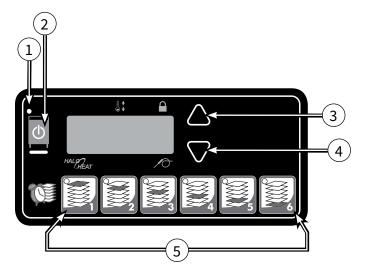
The shelf timers monitor food safety by using a first item in, first item out product management system. Holding times can be set for the products in each of the shelf positions. Products must be cooked to HACCP recommended internal temperature before being held in the holding cabinet.
