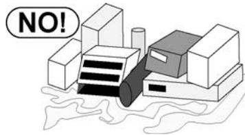
Make certain the indicator is not directly in front of a heating or cooling vent. Such a location will subject the indicator to sudden temperature changes, which may result in unstable weight readings.
