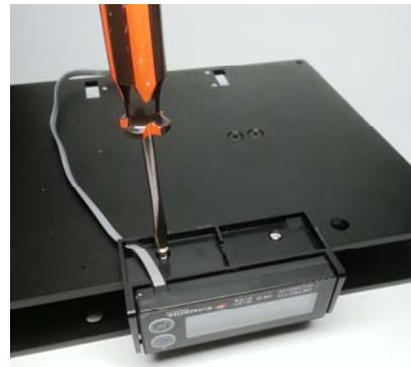
5. Route the cable into the scale and plug into scale display port (see interconnection section for port location and more information).
