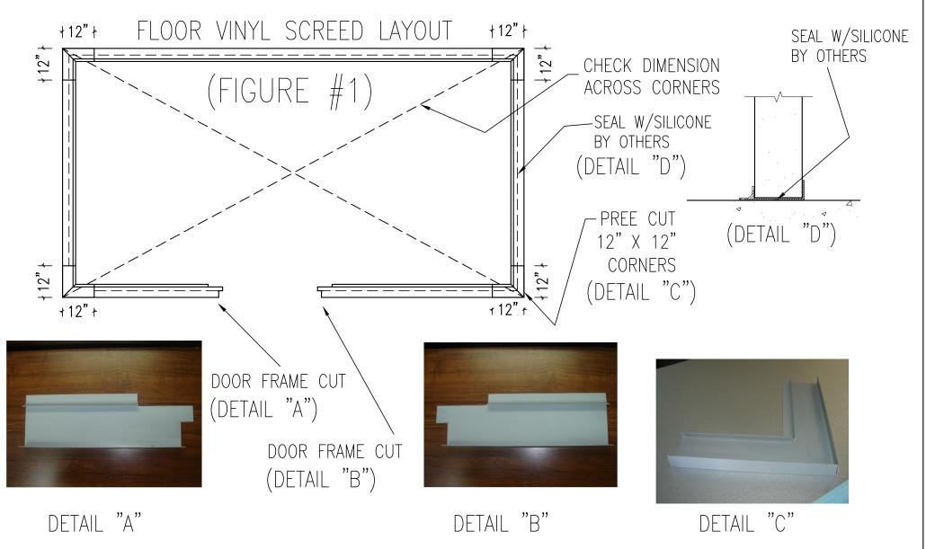
2-APPLY A BEAD OF SILICONE ALONG THE BOTTOM OF THE VINYL SCREED. THEN PLACE THE VINYL SCREED ALONG THE CHALK LINES.
