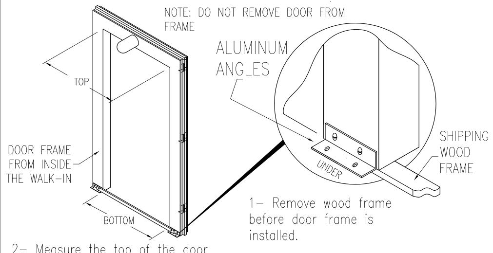
2— Measure the top of the door opening and measure the bottom of the door opening to make sure both measurements are equal.
