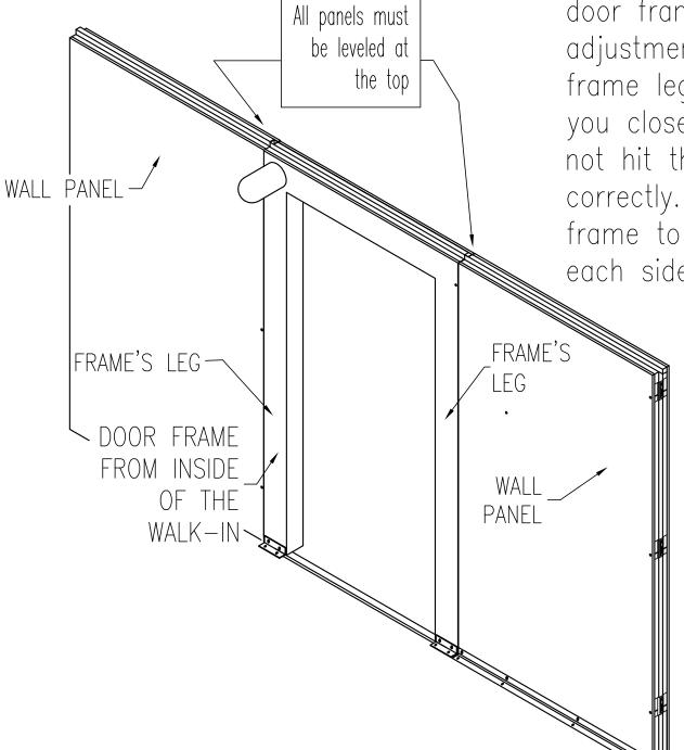
3— If the measurements are different, unfasten the cam—locks of the panels and on top, left and right side of door frame. then make necessary adjustments by pushing out the frame legs enough to ensure when you close the door, the door does not hit the frame and closes correctly. Then, secure the door frame to the adjacent wall panels on each side.
