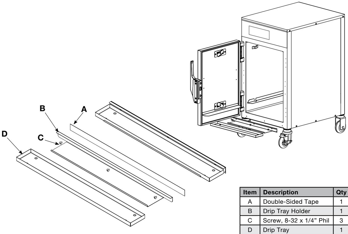
1. Poke holes through double-sided tape **A** which is attached to the back of drip tray holder **B**.
