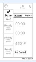
At the end of the cooking process, the oven sounds an alert and the chamber light flashes. The DONE screen displays.
