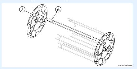
**Load** the spits one at a time and as evenly spaced as possible. This is done to maintain balance within the rotisserie.
