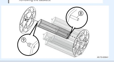
8. **Load** the baskets one at a time and as evenly spaced as possible. This is done to maintain balance within the rotisserie.
