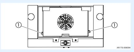
6. **Spray** Combitherm™ Cleaning Liquid inside of the fan convection box. Allow the cleaner to soften the grease for 10 minutes.
