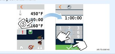
6. **Touch** the hold temperature setting **(6)**. **Enter** the hold temperature using the number pad.
