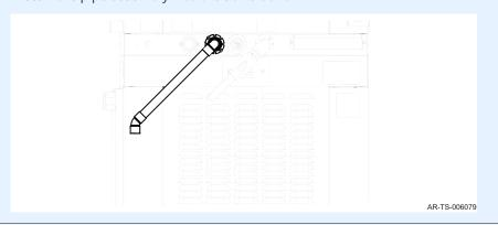
7. **Cut** a piece of pipe to a length that places the end of the pipe below the bottom of the oven.
