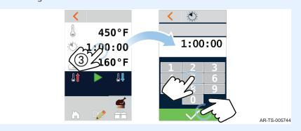
4. **Touch** the hold temperature setting **4**). **Enter** the hold temperature using the number pad. **Touch** the green check mark.
