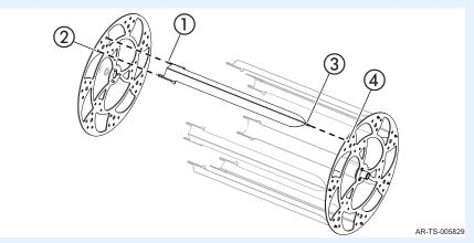
3. **Insert** the tapered, ridged-prong end ③ into the top hole ④ on the opposite side.
