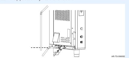
8. Run additional drain pipe to the floor drain.
