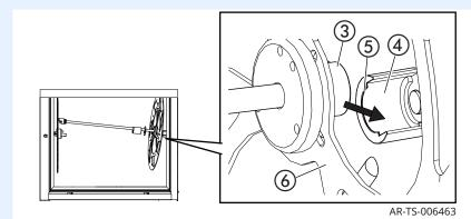
**Be sure** that the lip 5 of the cup is installed between the bushing and the disc 6.
