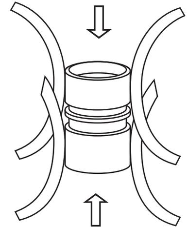
**3. Sandwich the Plastic Joint Between the Top and Bottom Brackets Firmly**
