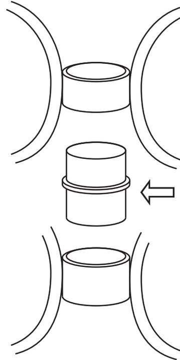
**2. Place the Plastic Joint Between the Top and Bottom Brackets**
