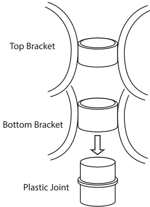
**1. Pull Out the Plastic Joint From the Bottom Bracket**
