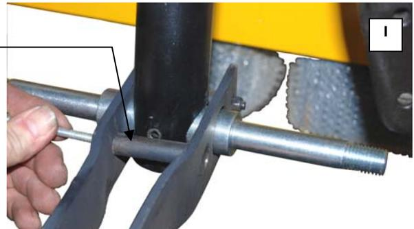
Step 5: Fix the wheel shaft in place.
