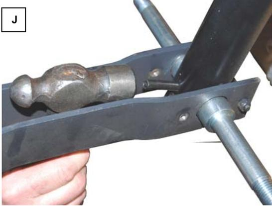
J. Rotate the wheel shaft until the hole for the retaining pin aligns with the opening in the steering shaft; then tap the retaining pin into place.
