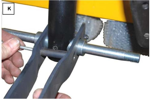
Step 6: Reconnect the wheels to the wheel shaft, by reversing the procedure described in Step 1 on p. 1.
