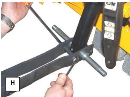
**I.** Remove the bolt and nut that fix the cross-link in place, and then remove the cross-link.
