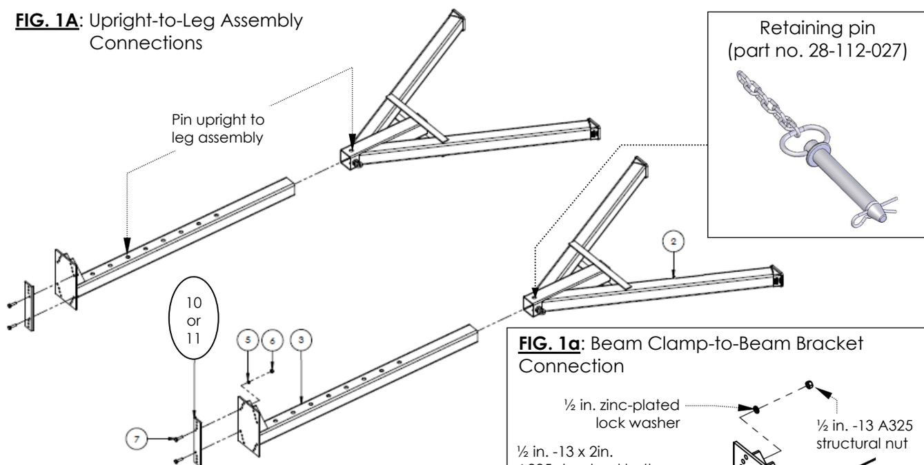
**FIG. 1a:** Beam Clamp-to-Beam Bracket Connection
