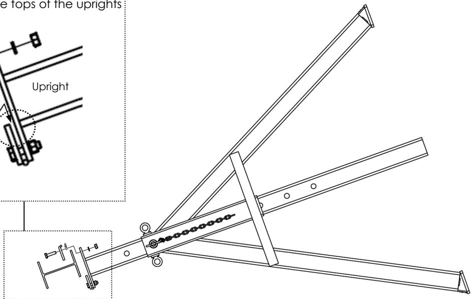
**FIG. 2C:** Exploded Parts View of Beam Clamp Connection to Beam
