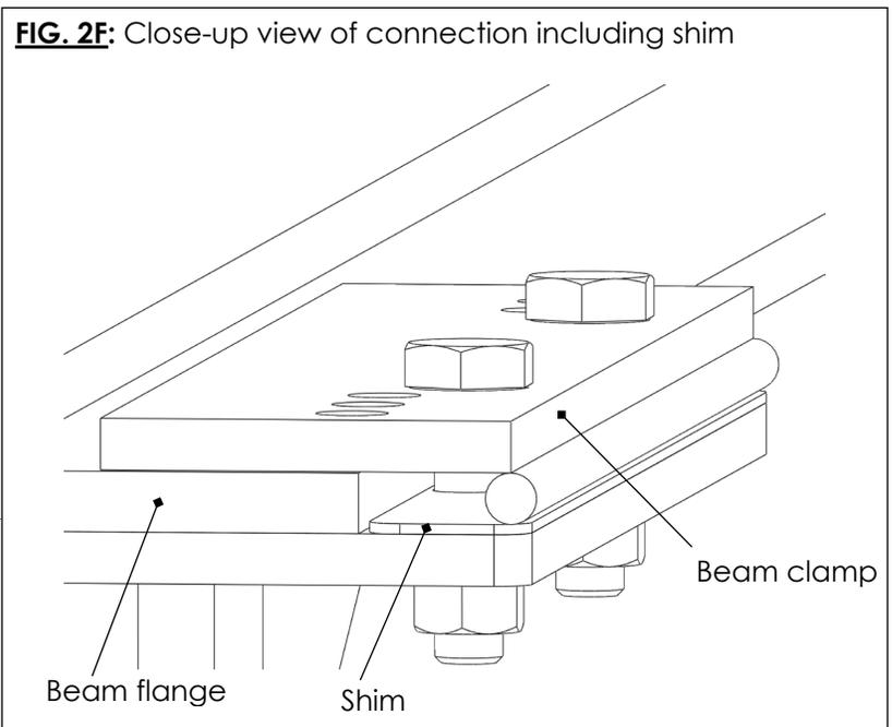
**Step 3:** Tighten the beam clamp fasteners to 50 - 52 ft·lb of torque.
