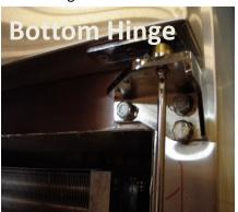
5) Using your wrench we recommend that you remove the top bolt & top hinge prior to removing the bottom. Note: You will need a second person to hold the door in place while you remove the bolts and take off the top hinge
