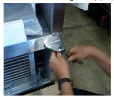
8) You will need to set the new bottom hinge (part# 178HINGABL) to full open, it must spring closed clockwise for door to close properly. Once the hinge is set, install the new bottom hinge.
