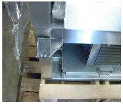
9) Place the spacer onto the bottom hinge and place the door onto the spacer. Once the door is on the bottom hinge correctly, close the door.
