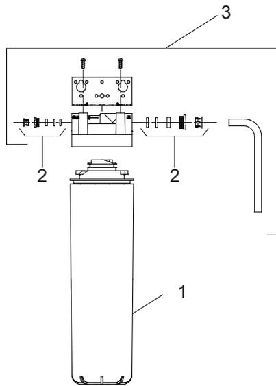
**Figure 9 - Filter Assembly**
