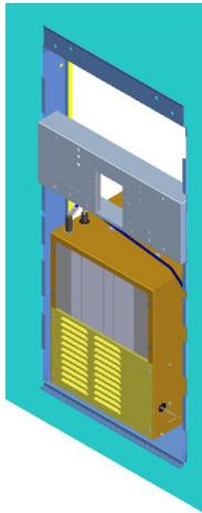
**Figure 2 - Chiller Installation**
