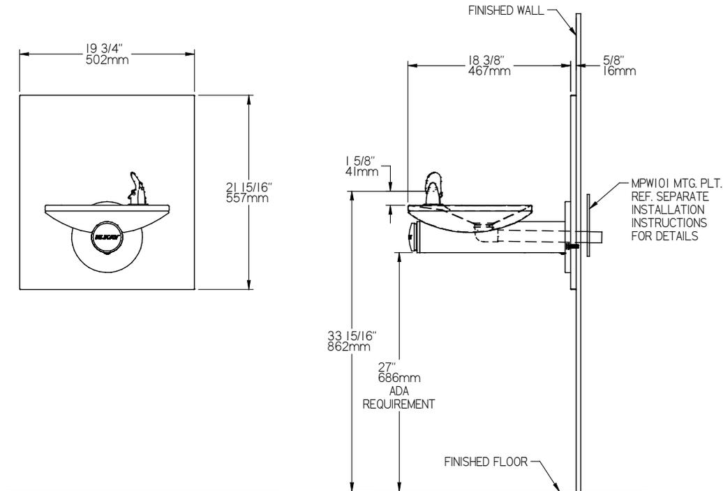
**Figure 6 -Rough-in Assembly EDFPB(V)114C W/MPW101 MOUNTING PLATE**
