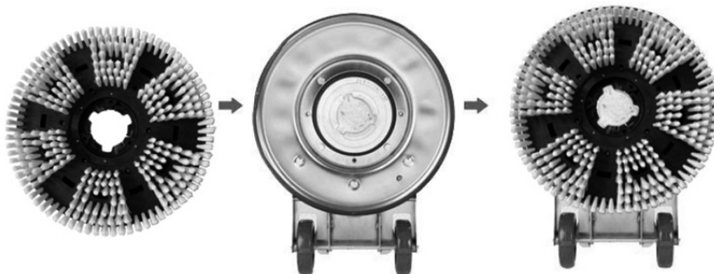
7) Align the disc brush with the bottom clasp and rotate it anticlockwise to fix it
