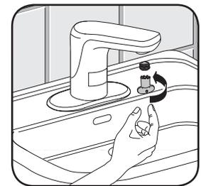
6. Install outlet and tighten with outlet key (supplied).
