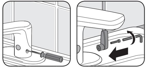
1. With a screwdriver, remove the round tab on the side of the faucet.
