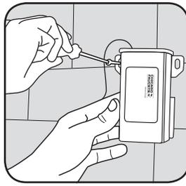
3. Insert anchors into holes and mount LTPS unit to wall with supplied screws.
