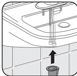
3. Below sink, feed hoses through large opening, and threaded mounting rod through small opening of deck flange. Deck flange should sit securely against underside of sink. For AC and LTPS take care not to pinch wire.
