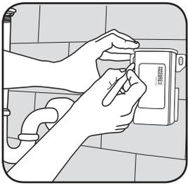
1. Position LTPS unit on wall and mark mounting holes on mounting surface.
