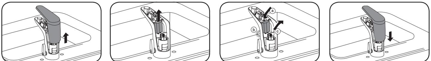
1. Loosen screw on underside of spout with allen wrench and remove cover.
