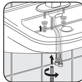
4. Place nut onto mounting rod and tighten with wrench.
