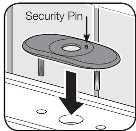
1. Mount cover plate if required. Use silicone caulk to seal plate to the sink. Security pin should be on the right side.
