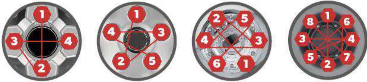
Figure 7-1 Lug Nut Sequence of Tightening
