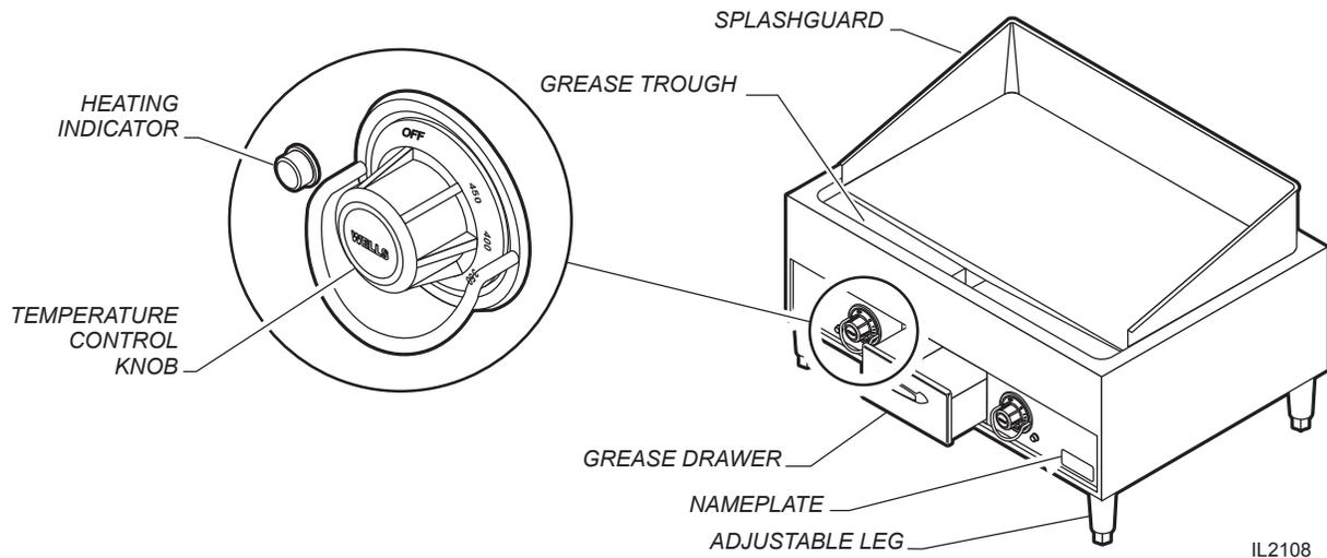
Fig. 1 Countertop Griddle Features & Operating Controls
