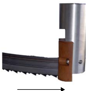
Figure 1: Direction of movement of band
