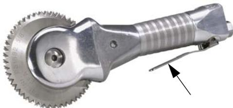
The air dehider is provided with a valve lever for regulating the compressed air current.
