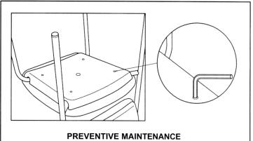
From time to time, check to make sure screws are securely tightened. Delta Holes in Plastic Seat Cover allow for convenient checking.
