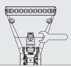
The jet nozzle can be removed with a 1/2" wrench.
