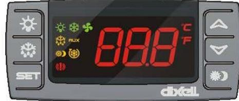
**SET**: To display target set point; in programming mode it selects a parameter or confirm an operation.
