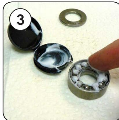
Install the bearing open side up. Apply a small amount of IKV-Fluor grease
