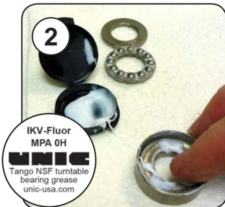
Place the lower race (groove up) in the cup and apply a small amount of grease
