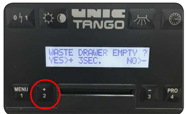
Press and Hold + for 3 seconds to start the rinsing cycle
