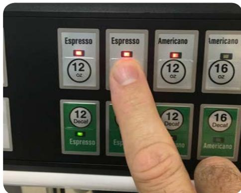
Press Single or Double to run a test cycle
