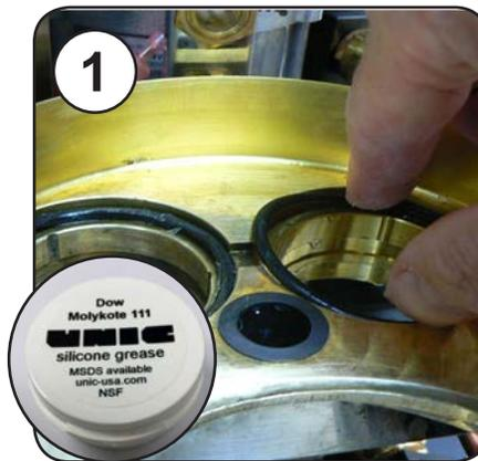
Install new O-rings with Molykote 111 grease
