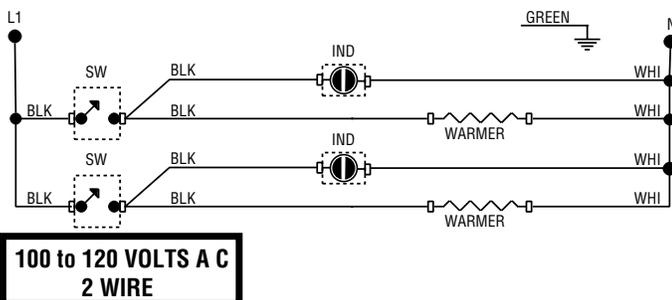
**SCHEMATIC WIRING DIAGRAM WX2A**
