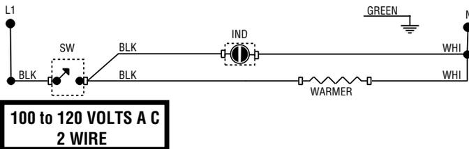
**SCHEMATIC WIRING DIAGRAM WX1A**
