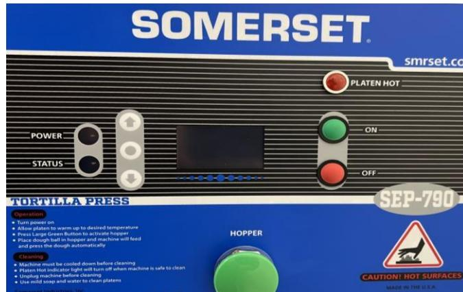
The SEP-790 is an electric tortilla press with heated top and bottom platens. The temperature of the platens and the press time are configurable through the main menu, which can be accessed from the default screen by pressing any of the menu buttons while the home screen is active. A slider at the bottom of the machine controls the gap between the platens.
