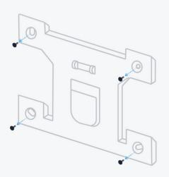
02 Align and snap the unit in place
