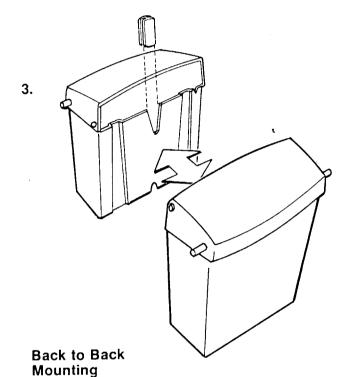
Hold two bases together at back, with liners removed, slide connector down over center slots.
