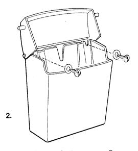
Place container on bottom screw. Remove liner and install top screws.
