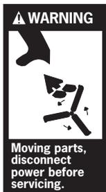
**WARNING: FAN IS GUARDED ON INTERIOR. EXTERIOR SHOULD BE MOUNTED AT LEAST 2.5 METERS ABOVE GRADE LEVEL OR PROPERLY GUARDED FROM ACCIDENTAL CONTACT OF THE BLADE THROUGH THE LOUVERS.**
