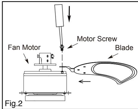
**NOTE: All set screws must be checked and retightened where necessary, before and after installation.**
