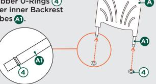
Begin installation by aligning Metal Tubes that protrude from the Backrest (A) with the opening of the Stool Frames (C).
