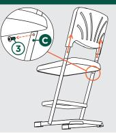
Double check all Bolts to be tightened securely before use. Check all Bolts periodically. Failure to completely tighten the Bolts may result in tipping and possible injury!
