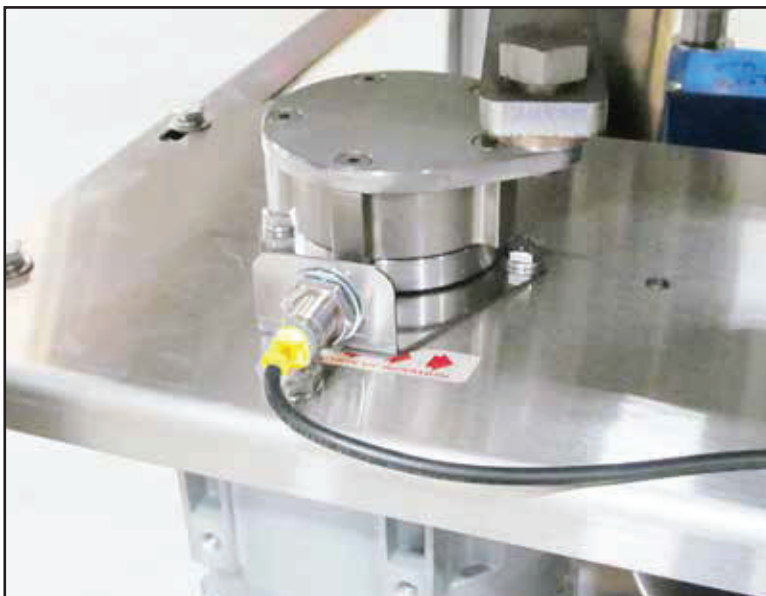
Fig. 24 - Clutch rotates counter-clockwise.
