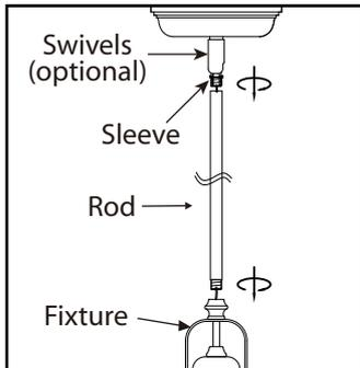
1. Install the length of rod that is required by threading wire through the rod and screwing it to the fixture. Install swivel to the rod, ensuring that the sleeve is at the swivel.
