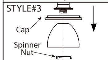
**Style#3:** Remove spinner nut from socket. Position glass on lamp and secure with spinner nut.
