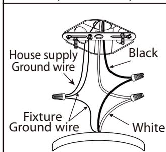
4. Once connections of wires are completed, carefully tuck wires and wire nuts into the outlet box making sure no bare wire (on the black and white) is visible at the wire nuts.
