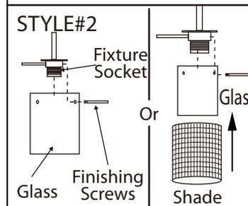
**Style#2:** Remove the finishing screws that are already on your fixture. Position glass in place and secure with finishing screws.
