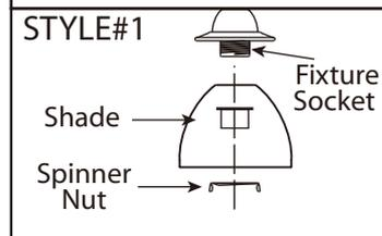
6. **Style#1:** Remove spinner nut from socket. Position shade on lamp and secure with spinner nut.
