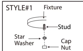
5. **Style#1:** Tuck electrical wires into electrical box and position fixture over studs on mounting bracket assembly. Secure fixture in place with star washer(s) and cap nut(s).
