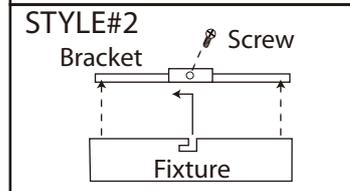
**Style#2:** Insert one screw into the mounting bracket - do not tighten yet. Tuck electrical wires into outlet box and position fixture over the mounting bracket. Line up the screw in the bracket to the "7" hole on the fixture. Slide fixture to secure in place. Insert remaining screw. Tighten both screws to secure.
