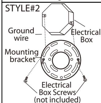
3. Connect the ground wires (bare copper or green) from your fixture to the ground wire (bare copper or green) or ground screw in the electrical box. Connect the black wire from the fixture to the black wire in the electrical box and connect the white wire from the fixture to the white wire in the electrical box.
