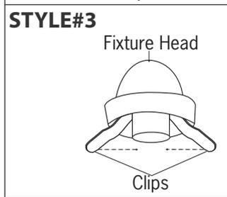
**STYLE #3** - Squeeze the two clips together around the socket. Slide the glass over the clips, then push the glass up snug to the fixture head.
