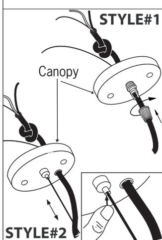
3. **Adjusting the length of flexible cord. For safety, do not release the knot inside canopy.**
