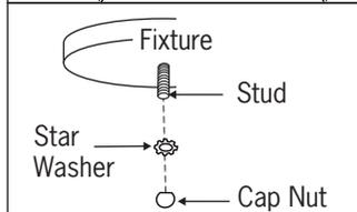
5. Once connections of wires are completed, carefully tuck wires and wire nuts into the outlet box making sure no bare wire (on the black and white) is visible at the wire nuts. Install the light fixture to the wall by aligning the hole(s) in the fixture with the studs or nipple on the mounting bracket. Secure in place with cap nut(s) and star washer (s).
