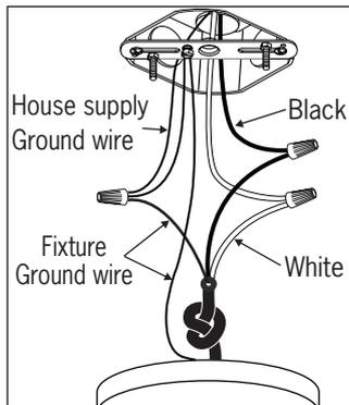
4. Firmly attach the fixture ground wire (bare copper) to the mounting bracket with the ground screw (by wrapping around the ground screw) and then connect it to the house supply ground wire with a wire nut. Connect the black wire (or wire marked "SPT-1") from the fixture to the black wire in the electrical box and connect the white wire from the fixture to the white wire in the electrical box.
