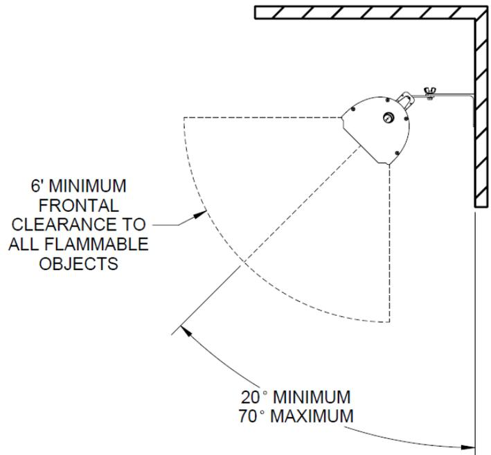
The angles of attachment are 20° to 70°, measured from the mounting wall.
