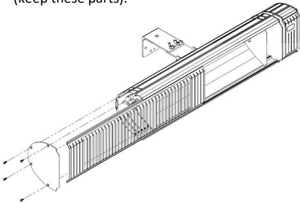
4. Carefully slide the protective grille out of the heater body to expose the emitter and the plastic sealing connectors.
