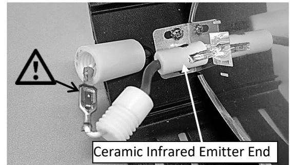
6. Bend the metal tabs to remove the small reflector shield sheet metal parts. Hold on to these pieces. This will allow you to slide the emitter into a bigger cavity to remove it from the reflector and heater body. Properly dispose of the broken emitter at your local recycling center.
