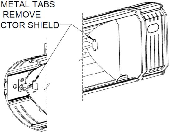
7. Hold the new emitter by the ceramic ends or wear clean dry gloves to prevent and position the new lamp inside the unit.
