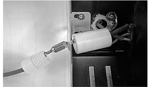
10. Carefully replace the protective aluminum grille and screw the protective end cap in place.
