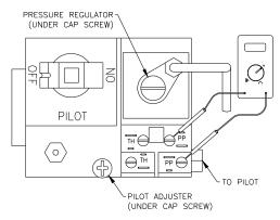
Note: Allow 3 to 5 minutes between flame adjustments to allow the reading to stabilize.
