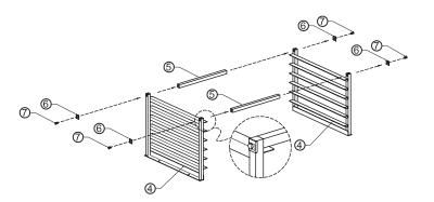
Connect the 2 ends of the rack together using the included posts and hardware
