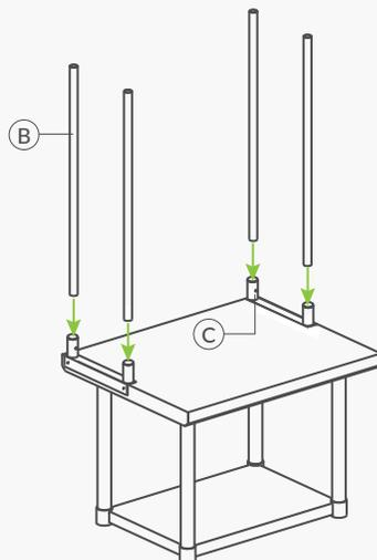
3. Add the overshelf top (D) and secure the legs into the gussets with the set screws (C). You may need to loosen a set screw if one struggles to go in.
