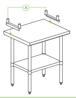
2 Secure the four legs (B) to the L-brackets using the Allen wrench and set screws (C) provided.
