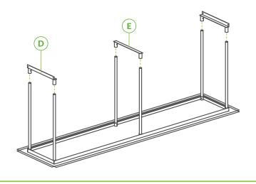
Align the overshelf to the back of the table to be mounted. Ensure the L-brackets are aligned properly and pre-drill holes through the side of the tabletop for screws. Screw L-brackets into the table (screws not included).
