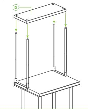
Add the overshelf top (E) and secure the legs into the gussets with the set screws. You may need to loosen a set screw if one struggles to go in.
