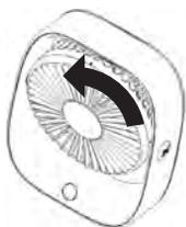
Make sure the fan is off. Open the front grill at anti-clockwise direction, take the front grill off.
