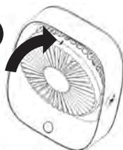
After washing, follow at clockwise direction to assemble the front grill back.
