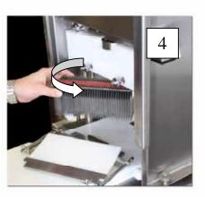
Slide the blade unit. Put it in a safe place.
