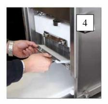
**5** Lift the plexi hood +/- 1cm. Up and push the latch backwards. **Hold the plexi hood** while still pulling the latch backwards and let the hood slide delicately down towards the stops.
